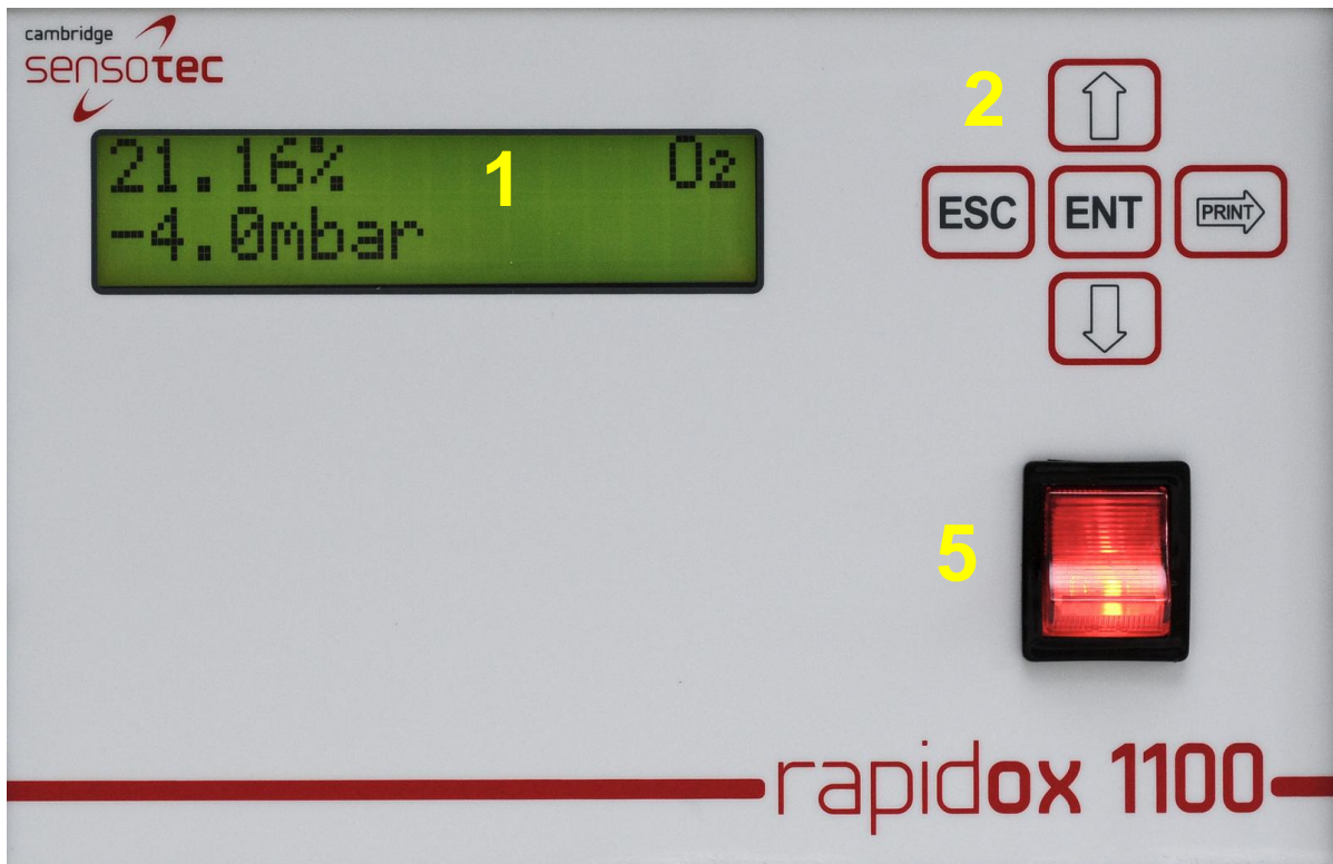
Figure 1: Rapidox 1100ER front panel. Numbers are referred to in the text.
