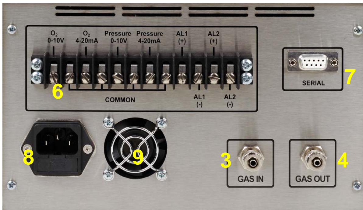
Figure 2: Rapidox 1100LR rear panel. Numbers are referred to in the text.
