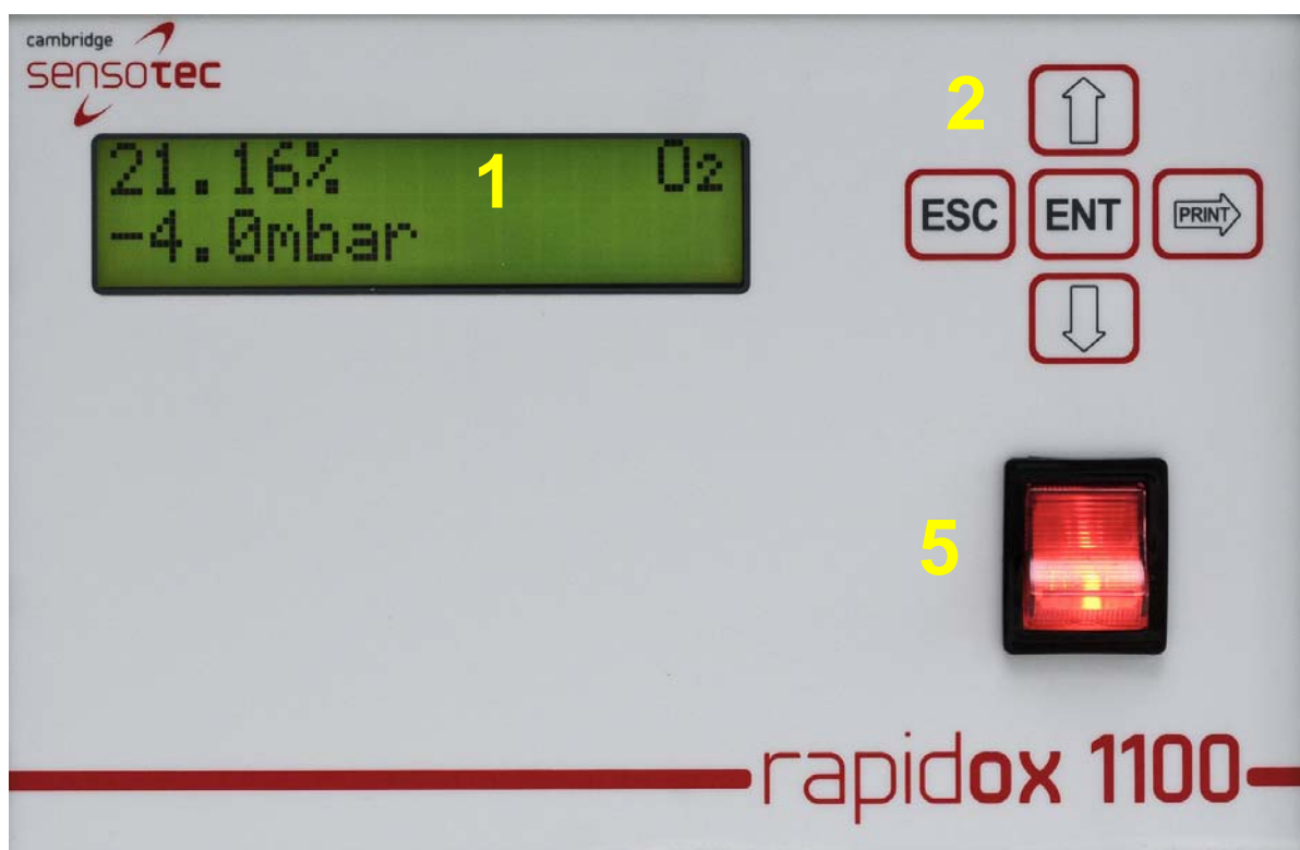
Figure 1: Rapidox 1100LR front panel. Numbers are referred to in the text.
