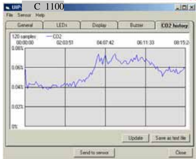
Figure 5. Example of a 8 hours working day recording extracted from the SenseAir Alarm unit using UIP-P
