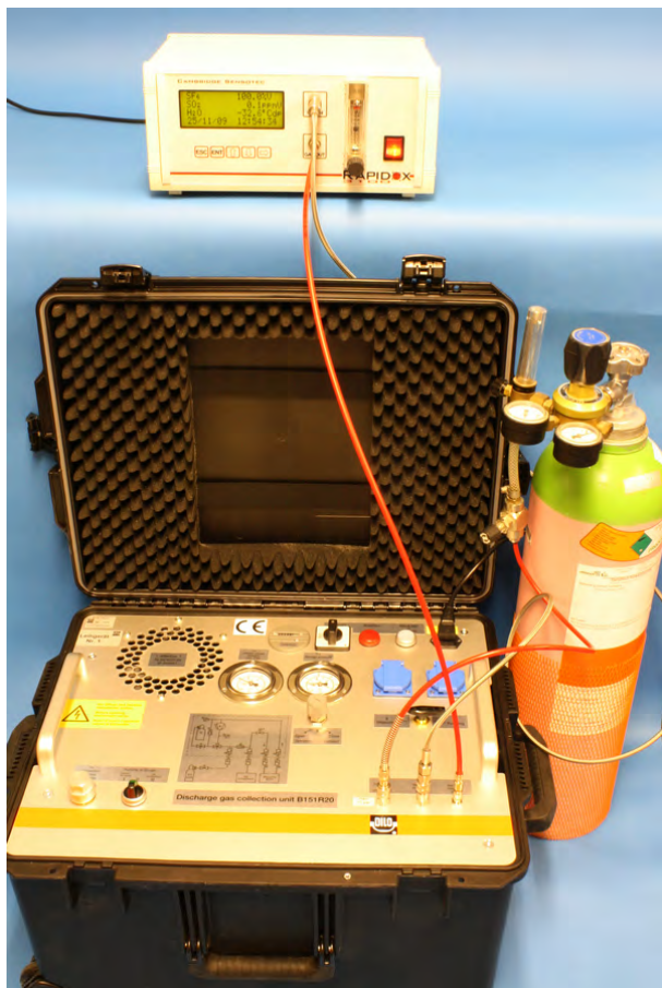
Rapidox Multimeter used in conjunction with a DILO Gas Recovery unit
