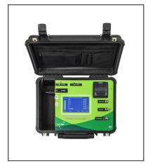
An optional pump enables two modes of operation. For samples that are taken from a gas source at atmospheric pressure or below, the pump is activated to draw a sample through the analyser. Alternatively, the pump can be deactivated when sampling from a source at a greater atmospheric pressure, allowing the gas to flow through the analyser. Gas flow is regulated manually via a rotary knob on the fascia and displayed electronically on the screen.
