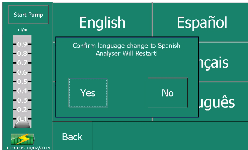
Figure 43: The analyser will ask you to confirm you really want to change the language before performing a re-boot.
