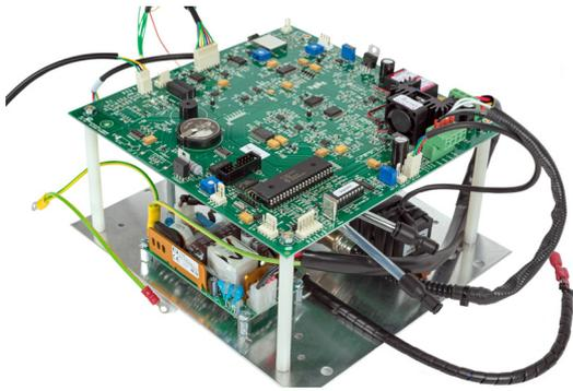
Specifically designed to measure ppm measurements in the 0-30% oxygen range at ambient temperature, the gas sample is pumped through the sensor via a tube allowing the unit to be located some distance from the measurement point.
