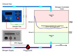
The inbuilt PFC (Proportional Flow Control) has been developed specifically to control the flow of inert nitrogen gas into the solder reflow oven very precisely. The analyser uses PID control theory to allow the readings from the Rapidox to make continuous adjustments to the valve to regulate the oxygen levels in the oven very precisely. The PID parameters are fully programmable to allow all types of oven sizes to be configured and controlled.
