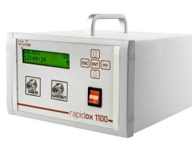
The Rapidox 1100J is a cost-effective argon gas analyser fitted with a durable thermal conductivity (TCD) sensor. The sensor is carefully heated to 50°C to prevent any ambient temperature changes causing drifting. Specifically designed to analyse argon purity in percent measurements, the Rapidox 1100J is ideal for applications such as welding, casting, titanium manufacturer, inert blanketing and glazing.
