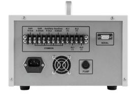
Configuration of the analyser allows for the instrument to be panel mounted with the gas fittings at either the front or rear.
