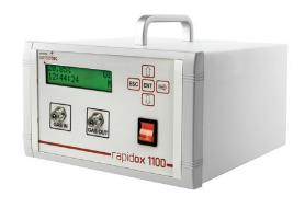
The Rapidox 1100Q is a cost-effective helium (He) gas analyser fitted with a durable thermal conductivity (TCD) sensor. The sensor is carefully heated to 50°C to prevent any ambient temperature changes causing drifting. Specifically designed to analyse He in percent measurements, the Rapidox 1100Q is ideal for applications such as gas generation, cooling, inert gas blanketing, leak testing, welding & diving.
