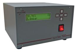
Zirconia oxygen sensors offer fast and accurate gas analysis over the low ppm oxygen range. They are particularly suitable for monitoring inert atmospheres and aggressive industrial applications within manufacturing processes.
