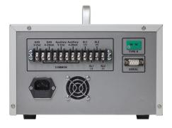
The temperature is determined either from the sensor head (up to 660°C) or above this, the temperature is recorded using the type K thermocouple which is fitted as standard.
